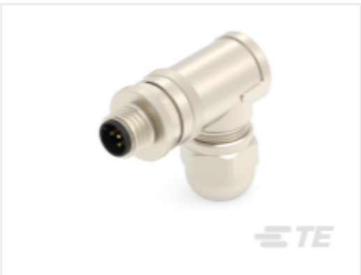
TE Part #T4113512051-000 M12 M, 5P GOLD D_CODE RA SHIELDED PG9
