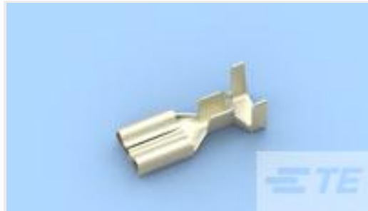
TE Part #1742899-1 187 FASTON,REC.,18-16 OR 2X18 AWG,NPST
