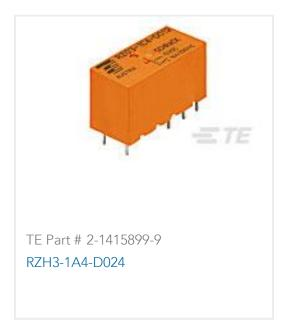
General Purpose Power Relay, DC, Monostable, 1 Form A SPST-NO, 16 A Contact Rating, 24 VDC Coil Voltage, SCHRACK Power PCB Relay RT1
