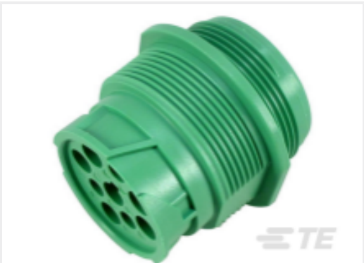
TE Part #HD10-9-1939P-BP03 REC, 9P, GRN,N, PANEL, J1939, TYPE 2
