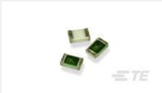
TE Part #3-1879223-2 CPF 0603 499R 0.1% 25PPM 1K RL
