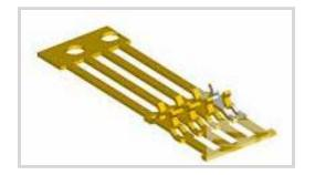
Leadframe Type: Single-In-Line (SIL) Centerline (Pitch): 2.54 mm [.1 in ] PCB Thickness (Accepted): .63 mm [.025 in ] Standoff Height: 1 mm [.039 in ] Leadframe Hold-Down Feature: Without
