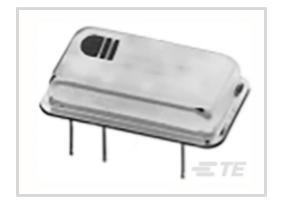
Input Current Type: DC Contact Arrangement: 1 Form A (NO) Input Voltage: 3.8 – 32 VDC Output Voltage Rating: 60 VDC Contact Current Rating: 2 A
