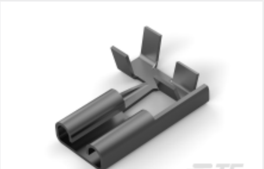
TE Part #4-280050-2 250 FASTON,FLAG,REC.,16-20 AWG, TPBR
