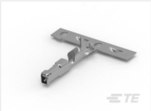
TE Part #2098762-5 Contact,female, 0.64, 20-22, CuNiSi, Sn
