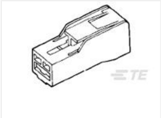
TE Part #172320-2 POSITIVE LOCK 250 (6.3 MM) HOUSING
