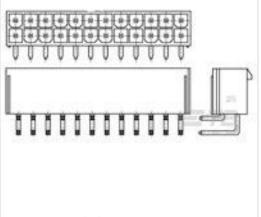
TE Part #1586041-4 4P VAL-U-LOK R/A HDR V2
