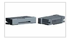
Centerline (Pitch): .5 mm [ .02 in ] Mating Retention Type: Zero Insertion Force (ZIF) PCB Mount Orientation: Right Angle Contact Mating Location: Bottom Termination Method to PCB: Surface Mount
