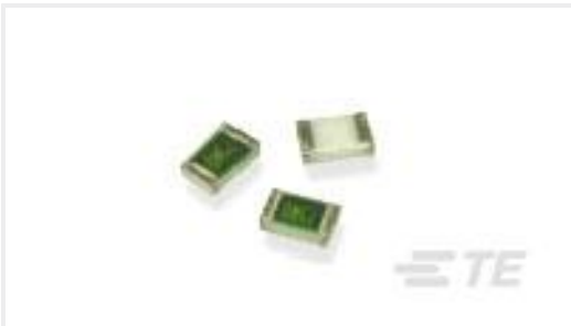
TE Part #1-1879134-2 RN 0603 12K7 0.1% 10PPM 1K RL
