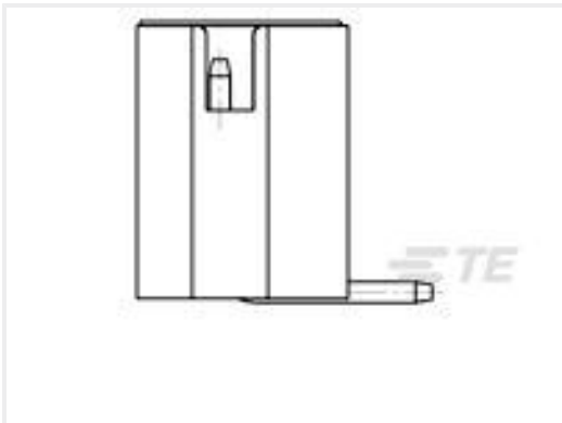
TE Part #1775317-3 HPL,2.5MM PITCH,V/T,SMT TYPE,3 POS
