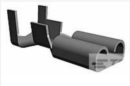
TE Part #170038-2 187 FASTON,REC.,20-16 AWG,TPBR
