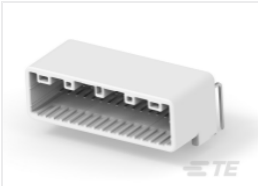
TE Part #2326784-1 32POS,TAB0.64X0.64,HDR ASSY, 90DEG,SLDR
