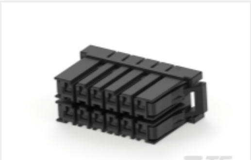
TE Part #CAT-D9934-A75B Receptacle and Tab Housing: 5.08 mm Pitch, 250-600V
