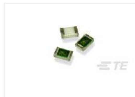
TE Part #6-1879208-6 CPF 0402 5K1 0.1% 25PPM 1K RL
