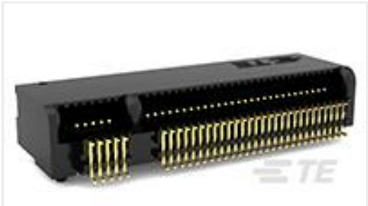
TE Part #1-2199230-6 M.2 0.5PITCH 4.2H KEY M 30U AU
