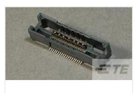
TE Part #2-5767004-2 MICTOR RECEPT ASSY, 38 POS.
