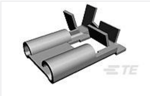
TE Part #63010-1 250 FASTON FLAG REC 18-14 AWG TPBR
