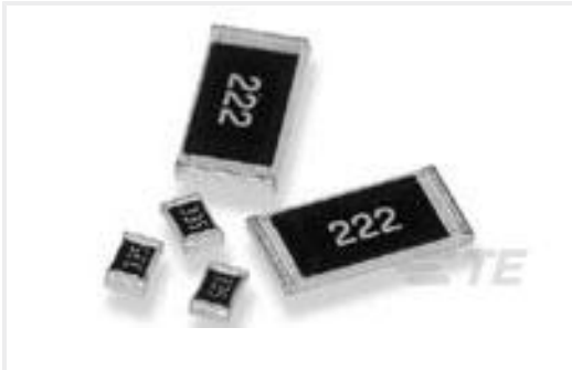
TE Part #1-2176186-6 CRGH1206 1% 2K2 0.5W
