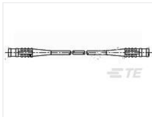
TE Part #1337815-1 50 OHM COAX SMB STR PLUG STR P
