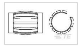
Contact Type: **Pin** Number of Positions: **1** Sealable: **No** Contact Current Rating (Max): **65** A
