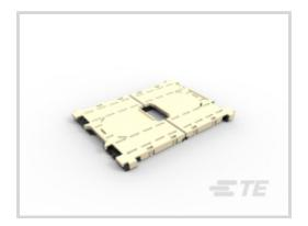
IC Socket Type: LGA 3647 Number of Positions: 3647 Contact Mating Area Plating Material Thickness: [30 µin] Centerline (Pitch): .86 mm, .99 mm [.034 in, .039 in] Termination Method to PCB: Surface Mount - Solder Ball
