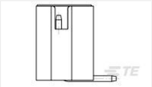
TE Part #1-1775317-0 HPL,2.5MM PITCH,V/T,SMT TYPE,10 POS
