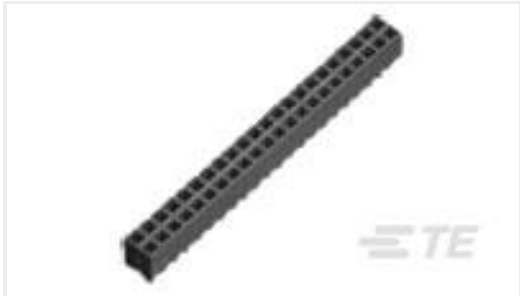
TE Part #4-1734506-4 RCPT, 2.0MM, 42P,VRT MT, 8 Au", 2.6 ST
