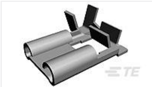
TE Part #63901-1 250 FASTON FLAG REC 18-14 AWG TPBR
