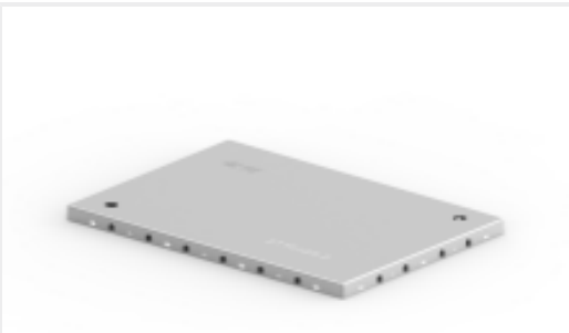
TE Part #2118729-2 STD SHIELD COVER, CRS-44.60X31.10X2.00MM
