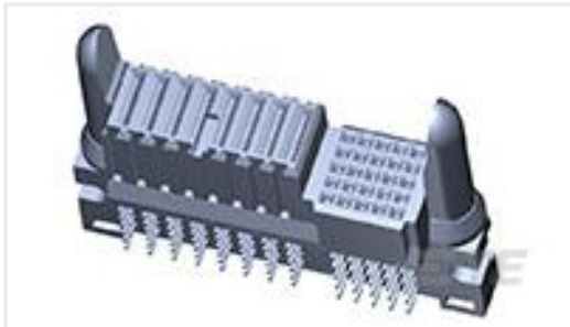
TE Part #2360871-2 56 POSITION SLIVER ORTHOGONAL EDSFF 1*1
