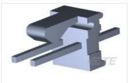
TE Part #641215-2 02P MTA100 HDR ASSY FL/ST 30AU PCB Mount Header, Vertical, Wire-to-Board, 3 Position, 2.5 mm [.098 in] Centerline, Fully Shrouded, Tin (Sn), Through Hole - Solder, Economy Power 2.5
