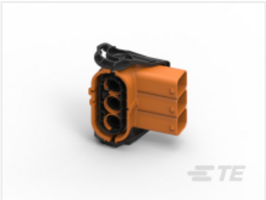
TE Part # 1-2141166-1 3POS,8MM HV,REC HSG,90DEG,ASSY, SEALED
