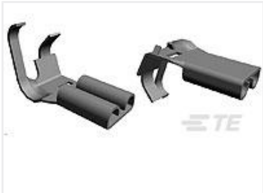
TE Part #42486-3 187 FASTON FLAG REC 20-16 AWG NPST
