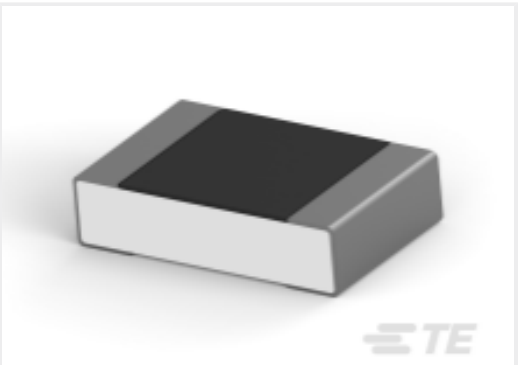
TE Part #2-2176382-7 RQ 0805 249K 0.1% 10PPM 5K RL
