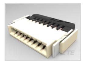
Centerline (Pitch): .5 mm [ .02 in ] Mating Retention Type: Zero Insertion Force (ZIF) PCB Mount Orientation: Right Angle Contact Mating Location: Dual Side Termination Method to PCB: Surface Mount
