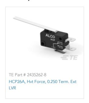
26 A Snap Action Switch, Single Pole - Double Throw Configuration (Pole-Throw), Extended Lever, 125 VAC / 250 VAC, 110 g [3.88 oz] Operating Force
