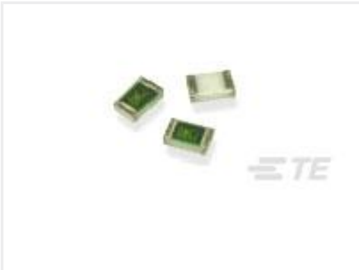
TE Part #1676294-3 RN 0805 2K74 0.1% 10PPM 5KRL
