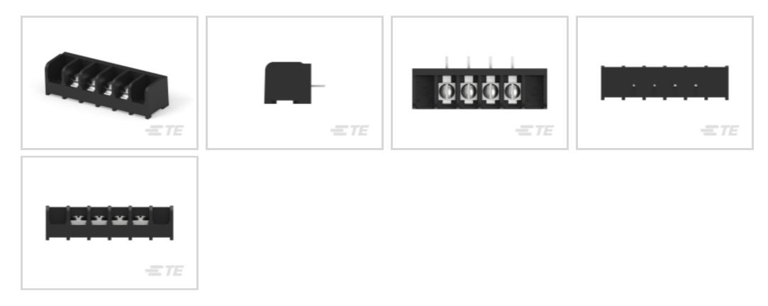
Number of Positions: 4 Barrier Strip Style: **Tri-Barrier** Bottom Termination Type: **Printed Circuit Pin** Connector System: **Wire-to-Board** Centerline (Pitch): **9.53 mm [.375 in ]**
