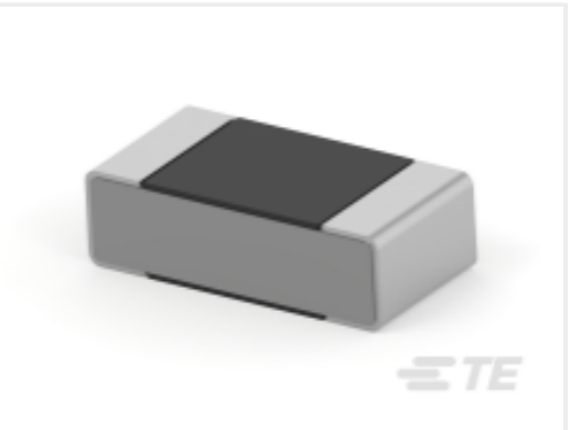
TE Part #1-2176280-7 CPF 0402 158K 0.1% 25PPM 1K RL
