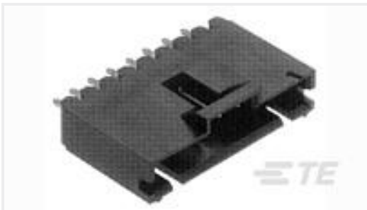
TE Part #103670-7 08 MTE HDR SRST LATCH W/HLDWN
