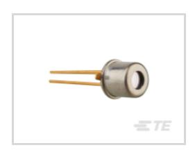
Optical Detector Type: Avalanche Photodiode
