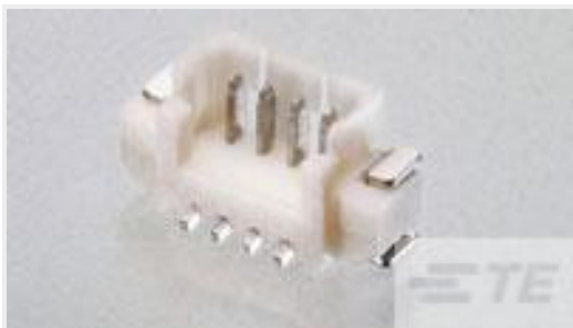
TE Part #1734260-4 1.25 WTB HDR SMT, 4 POS
