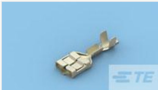
TE Part #2178438-1 250 FASTON,F-SPR REC.,24-20 AWG, PNST
