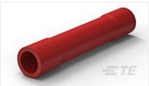
TE Part #34243 PG BUTT SPLC 22-16COMM22-18MIL
