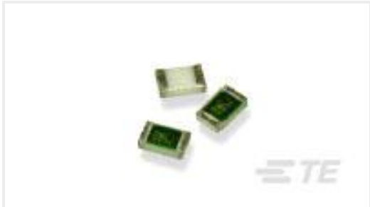
TE Part #2176216-1 CPF A 0603 10R 0.1% 25PPM 1K RL
