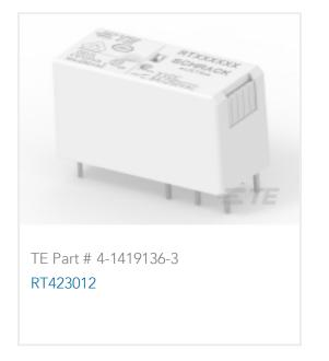
General Purpose Power Relay, AC, Monostable, 2 Form C DPDT-CO, 8 A Contact Rating, 230 VAC Coil Voltage, SCHRACK Power PCB Relay RT2
