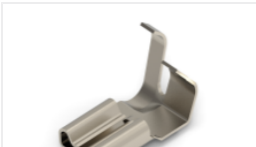
TE Part #1742543-4 250 FASTON,FLAG,REC.,18-12 AWG, NPST
