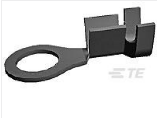
TE Part #40660 RING 164(4.17 MM) TERMINAL 18-14 AWG BR
