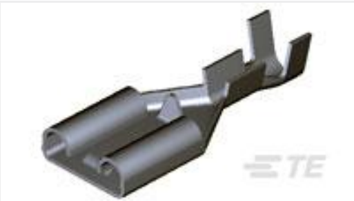
TE Part #63854-2 250 PL MKIII REC. 18-14AWG TPBR
