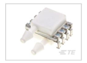
Pressure Sensor Type: Analog Pressure Sensor Modules Pressure Type: Differential Pressure: [2 inH2O] Proof Pressure Range: 300 psi Output Signal Type: 5-95% Vdc
